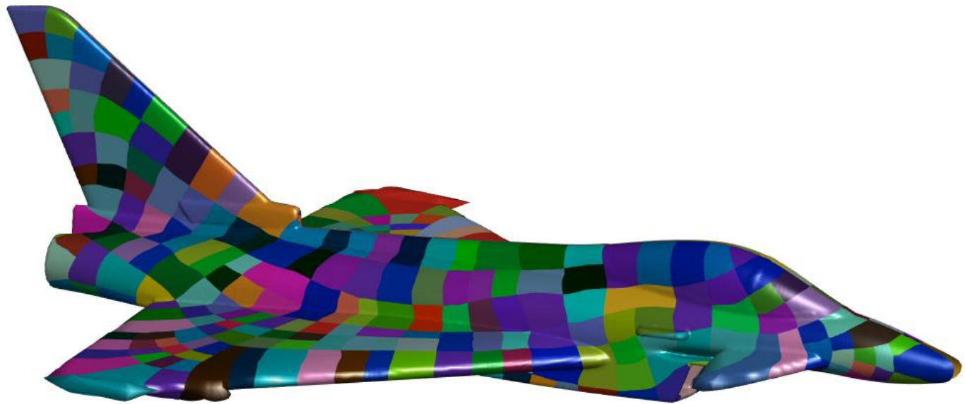
Fig. 14. Fighter jet model composed of 300 30 th -order discontinuous quadrilateral elements by the technique in Fig. 7.
