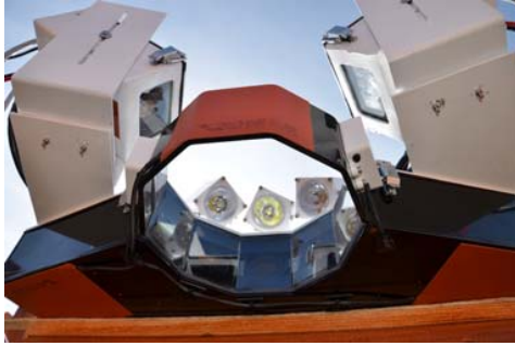
Fig. 2. Multi-Angle Snowflake Camera (MASC) at the MASCRAD Snow Field Site in Fig. 1.
