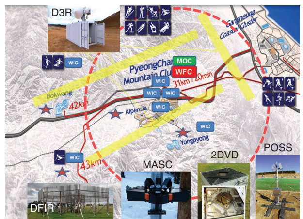
FIGURE 15. ICE-POP 2018 in South Korea, with a magnified picture of the Olympics venues, spread between the coastal area and the mountains. Some instruments at the main Mayhills supersite are shown (see the similarity with Figure 1) as well as NASA's dual-polarization, dual-wavelength ( K_u , K_a )-band radar (D3R) [25].
